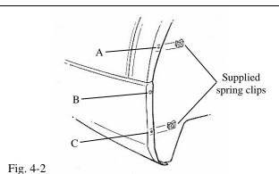
(b) Install supplied M5 spring clips over the panel edge dimple at locations A and C with the turned up edge on the inside of the panel (Fig. 4-2).
